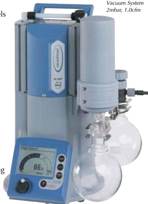
Low-profile outlet condenser reduces height requirements.
