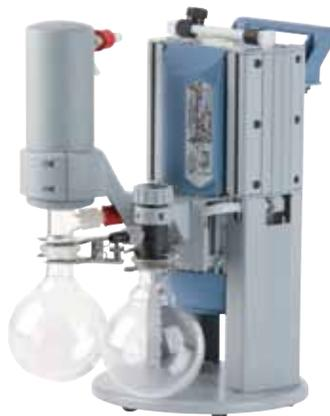
For SDS-PAGE concentrations greater than 10%, choose the MD1C+AK+EK. Its integral pump achieves deeper vacuum levels for enhanced evaporative performance, and the catchpots and condenser protect the pump and the lab atmosphere without the cost and inconvenience of a cold trap.
